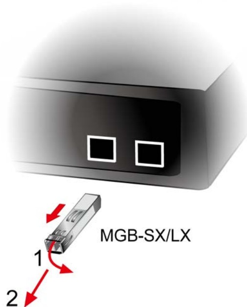
Figure 2-2-5: How to Pull Out the SFP/SFP+ Transceiver
