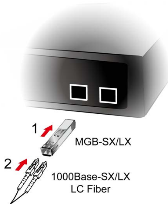
Figure 2-2-4: Plug-in the SFP/SFP+ Transceiver
